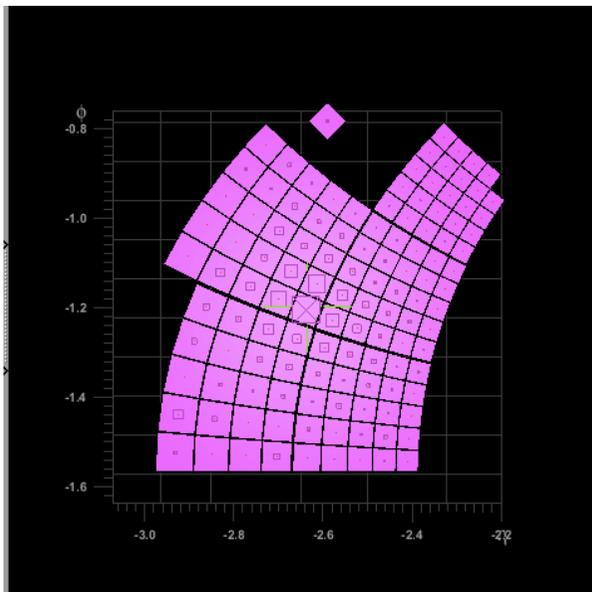
A noisy ECAL tower reconstructed as high pT photon can cause pT imbalance and unphysical MET distributions. The noisy events are identified and filtered.
